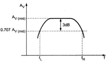
In figure shown, fL and fH are the lower and upper cutoff frequencies where the voltage or the current gain falls to 70.7% of the maximum gain. Bandwidth BW=( fH- fL).
