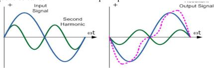
16. **Phase Distortion** or **Delay Distortion** is a type of amplifier distortion which occurs in a non-linear transistor
