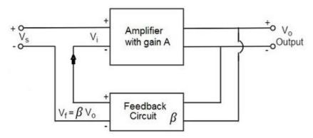
4. The gain of the amplifier is the ratio of output voltage Vo to the input voltage Vi. the feedback network extracts a voltage Vf =  $\beta$  Vo from the output Vo of the amplifier. This voltage is added for positive feedback and subtracted for negative feedback, from the signal voltage Vs. Now,
