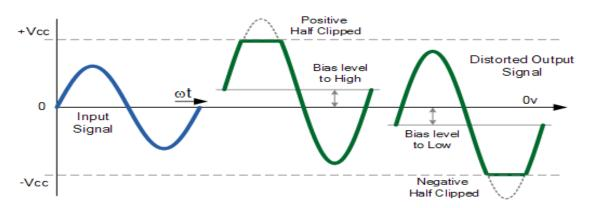
14. The output voltage signal becomes clipped in both the positive and negative parts of the waveform an no longer resembles a sine wave, even when the bias is correct. This type of amplitude distortion is called **Clipping** and is the result of "over-driving" the input of the amplifier.
